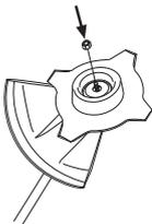
When fitting, tighten the nut in the opposite direction to the direction of rotation of the cutting attachment. To remove it, undo the nut in the same direction as the cutting
